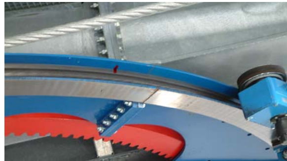
Method to check gliding of the bull wheel liner
