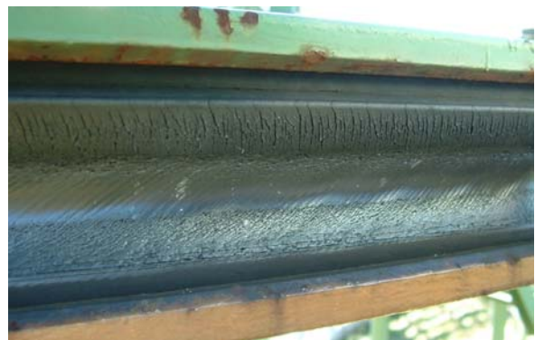
Thermal corrosion of bull wheel liners
