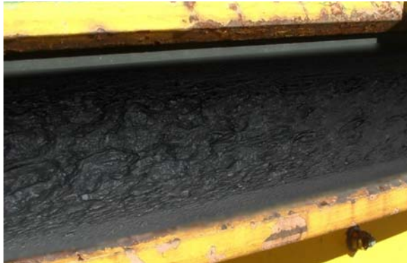
Typical damage of improper use of grease
